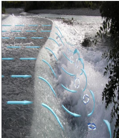
Weirs: A weir with animation showing the flow of water over the river
