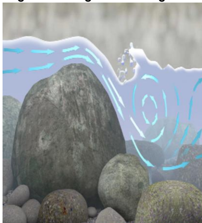
Re-circulation waves: Cross-section diagram showing re-circulating wave
